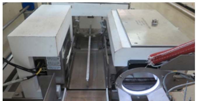
Figure 2: Image of a typical ex-situ inspection area. SNM packages rest on the central rail between the shielding blocks.
