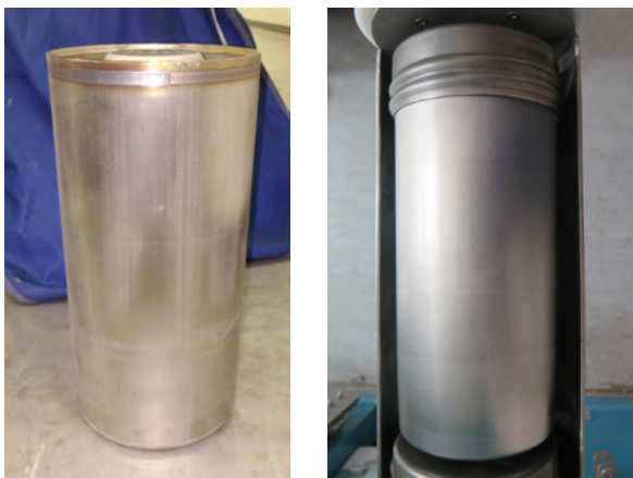
Figure 1: Images of typical SNM canisters, the left hand image is a welded SNM package and the right hand image is a screw-top 'overpack' SNM package.
